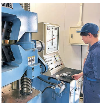
▲材料力学実験(鋳鉄の引張試験) Material strength test (Tensile test of cast iron)
